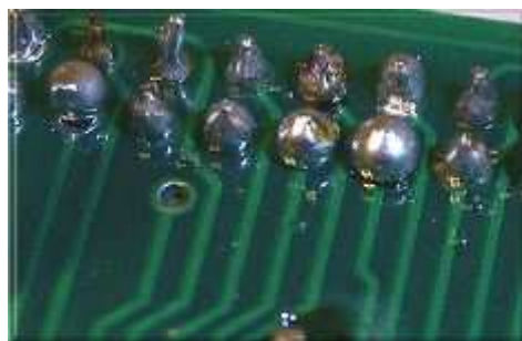
Figure 2 Bad Soldering ( http://www.epemag.wimborne.co.uk/desolderpix.htm )
