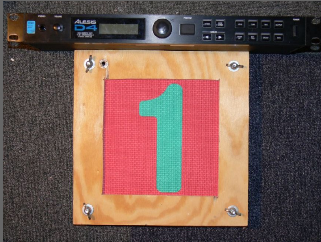
MIDI trigger interface / drum machine + custom piezo trigger pad
